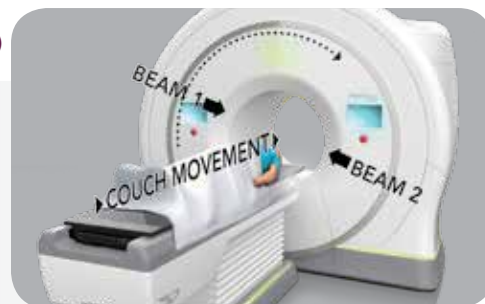
2 – 12 discrete gantry angles can be used in TomoDirect delivery mode
